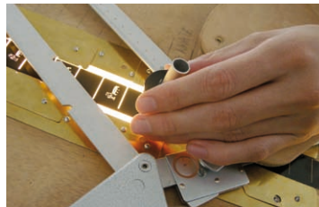
Pantograph: A unit to to enlarge or reduce plans or maps.
